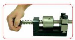
With the cover closed and the hose held in place begin rotating the wheel until it cannot rotate any further. Measure depth of nut to prevent overthreading.
