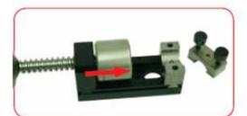
Release the hose clamp assembly by releasing the thumbscrews. Slide the socket nut holder open.
