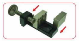
Unscrew the socket nut holder and screw on the vice adaptor.
