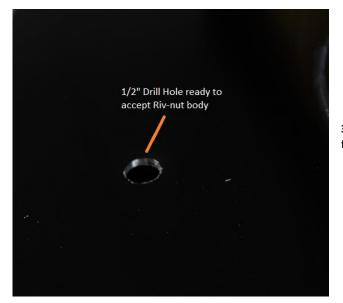
**3.** Drill out the hole and ensure to thoroughly clean up all metal shavings from the fuel tank and using a deburring tool to clean up the drill hole.
