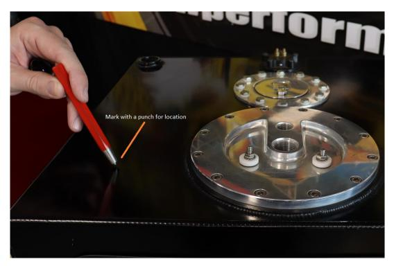
Using a drill and a 1/2" drill bit suitable for drilling metal. We recommend to drill a small pilot hole (with a smaller drill bit) first to preciously get the position required.
