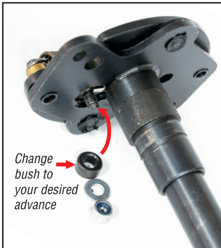
Figure 6 Changing the Advance Stop Bushing
