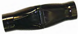
SCHOENFELD Knoxville Mufflers These mufflers are designed to control noise down to 100dba from 100 feet for 410 Sprintcars. Straight through design, 3-1/2" inlet and outlet. SCH-112535
